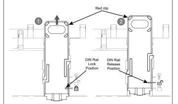
6. Hold the controller in an orientation such that the red clip is facing downwards and towards the DIN rail.
