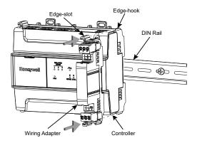
Mount the adapter in a way that the edge-slot of the adapter aligns with the axis of the edge-hook of the controller to attach and secure them together.
