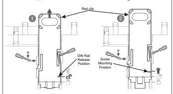
**NOTE:** Repeat step 5 of Mounting the controller on a wall or panel using Din rail in case the red clip is in the lock position.
