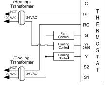
IMPORTANT: Before wiring, remove pre-installed RC/RH jumper.
